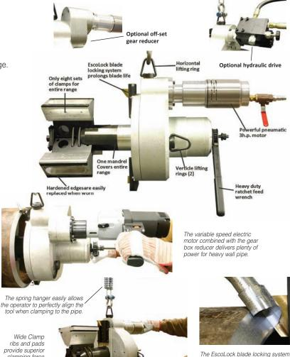
holds the blade securely in place to produce a thick chip that helps prolong blade life by transferring the heat to the chip and away from the cutting blade.
