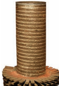
The tube is ready for end prepping after the fin is removed.
