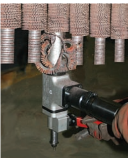
The Fin MILLHOG can remove a 4" fin from a tube O.D. in under two minutes and can be used in any orientation.
