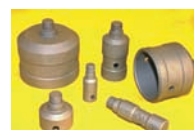
A properly sized Pilot is .015in - .030in under the i.d which is necessary for smooth operation, long blade life and chatter free bevels.
