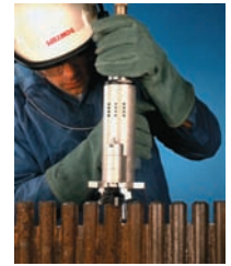
Both the HHB-5,000 and HHB-10,000 Straight Drive models can be hand held or track mounted.
