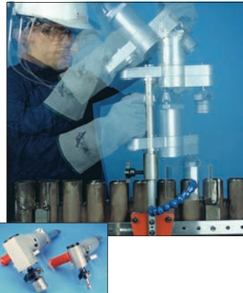
These high speed straight-thru hand held bevelers provide torque-free operation and feature quick-change tooling. Right angle models are available for getting into tight spaces.
